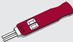
1. Remove the red sample collector from the white test cassette. **Do not remove the protective Cover. Do not touch the sampling pads.**
